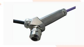
The ETK8...-Ex system is a very easy and fast to install connection kit, based on an approved screw technology. Our version with integrated ambient thermostat makes it possible to realize power supply, branch of heating cable and thermostat - all in one device! Direct switching capacity is up to 16A. Typical applications are simple frost protection applications on pipes, tanks, and heat jackets.
